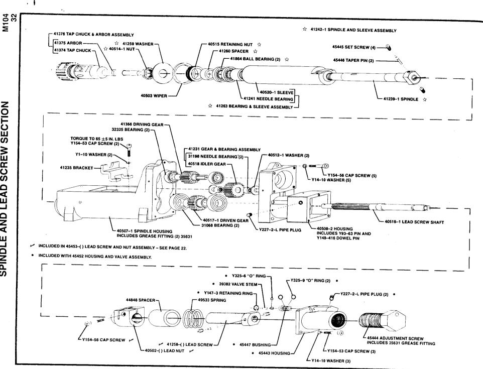
SPINDLE AND LEAD SCREW SECTION
